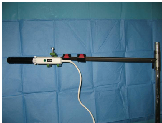
Figure 2 Ultraviolet A lamp held by a clamp mounted on an intravenous pole.
