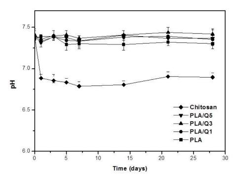
**Figure 5.** Changes in pH of PBS solution after different immersion times of PLA, chitosan, and PLA/chitosan composites with 1 wt % (PLA/Q1), 3 wt % (PLA/Q3), and 5 wt % (PLA/Q5) chitosan.
