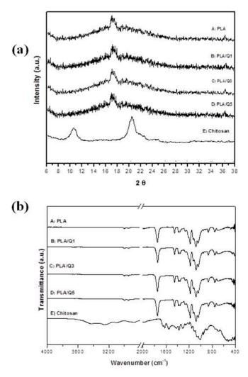
**Figure 3.** (a) X-ray diffraction patterns and (b) FT-IR spectra of A) PLA; PLA/chitosan composites with B) 1 wt % (PLA/Q1), C) 3 wt % (PLA/Q3), D) 5 wt % (PLA/Q5) chitosan, and E) chitosan.
