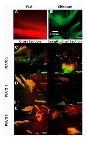
**Figure 1.** Confocal microscopy micrographs of **(A)** Polylactic acid (PLA), **(B)** Chitosan particles, and **(C–E)** PLA/chitosan composites. The PLA and chitosan particles show red **(A)** and green **(B)** autofluorescence, respectively.
