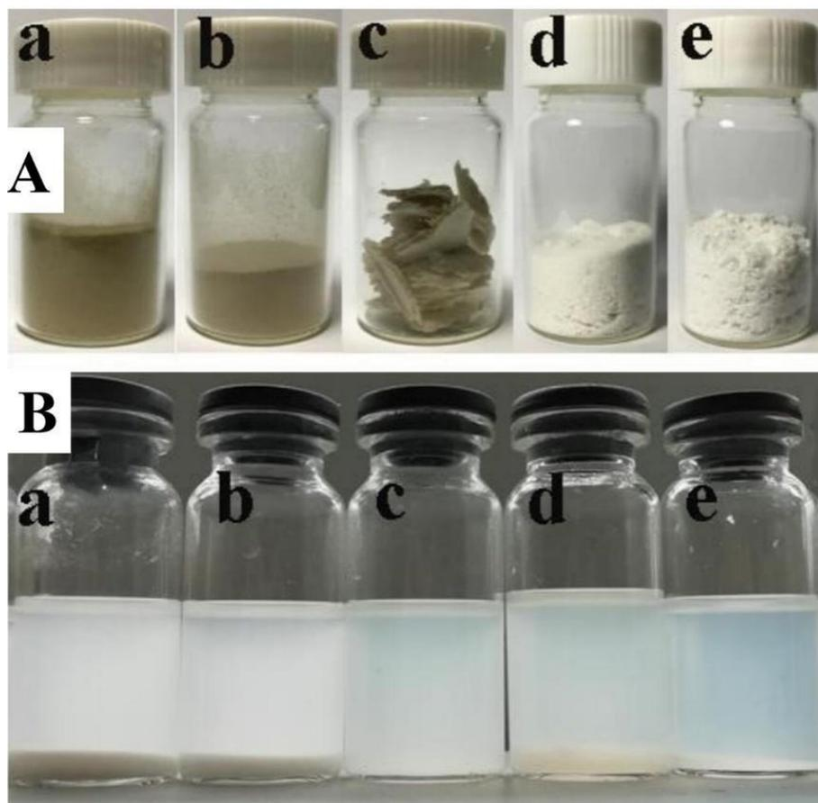
**Figure 8.** (A) Photographs of products from rice straw to RSCA at different stages: (a) rice straw powder, (b) pretreated rice straw, (c) rice straw-derived coarse cellulose (d) RSC, (e) RSCA. (B) Photographs showing the solubility property of RSCA with different DS: (a) DS = 0.51, (b) DS = 0.75, (c) DS = 1.12, (d) DS = 2.75, (e) DS = 2.82.
