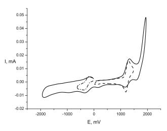
**Figure 5.** Cyclic voltammogram of complex **16** on the GC electrode (sweep rate 100 mV/s,  $C = 1 \times 10^{-3}$  M, n-Bu4NBF4, and rel. Ag | AgCl | KCl(sat.)).
