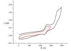
**Figure 4.** The cyclic voltammogram of complex **16** in the anodic range (sweep rate 100 mV/s,  $C = 1 \times 10^{-3}$  M, n-Bu<sub>4</sub>NBF<sub>4</sub>, and rel. Ag | AgCl | KCl(sat.)).
