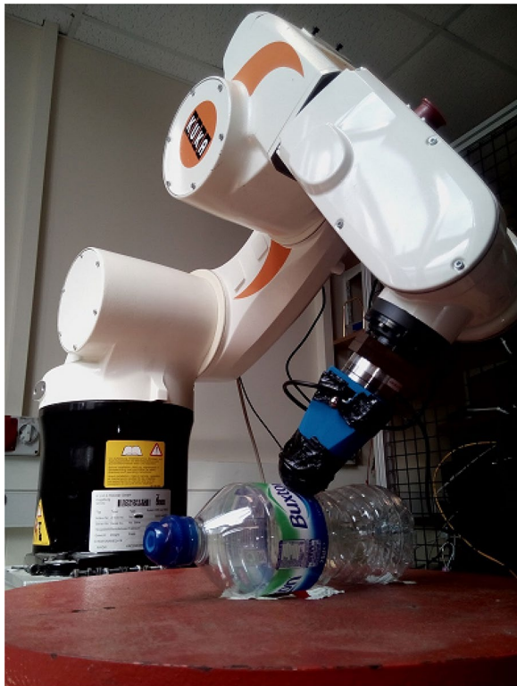
Fig. 1 Tactile data are collected autonomously by the tactile sensor developed in [7], mounted on a KUKA KR-650
