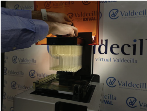
Figure 2. Test swabs manufactured on a Formlabs 3D printer. Figure taken with permission from Formlabs, 2020.
