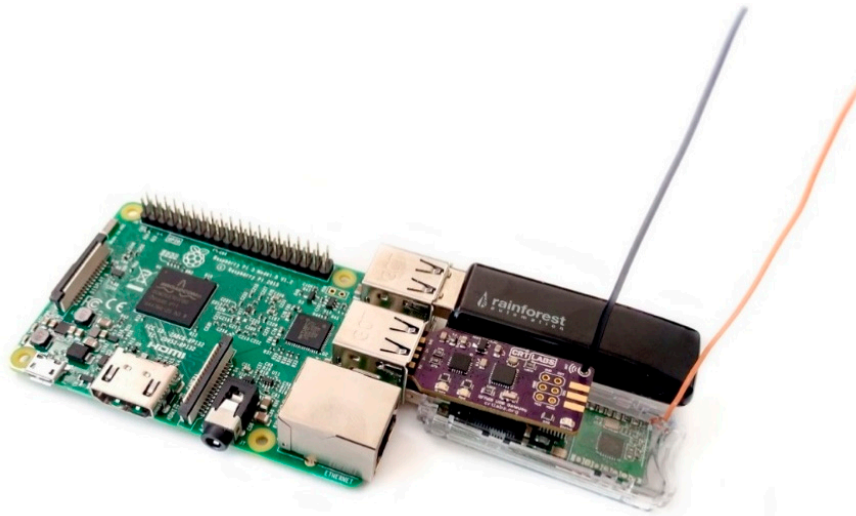
Figure 4. Raspberry Pi backhaul with gateways to connect with various wireless devices.
