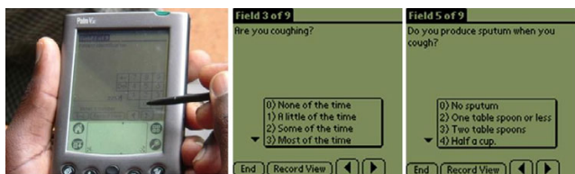
Figure 3 The programmed PDA and sample screens. A: PDA in use. B: Screen used to collect data on cough. C: Screen used to collect data on sputum production.
