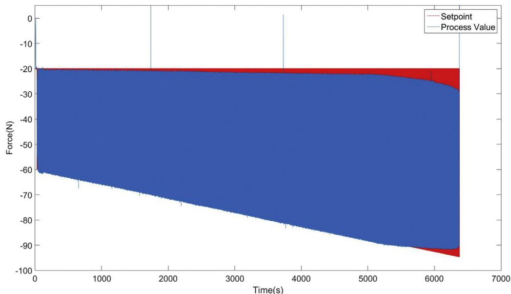
**Figure B.1** Load–time curve of specimens that sustained more than 30,000 cycles, in terms of set point of the command signal (red) and processed value (blue), indicating a good match between them.
