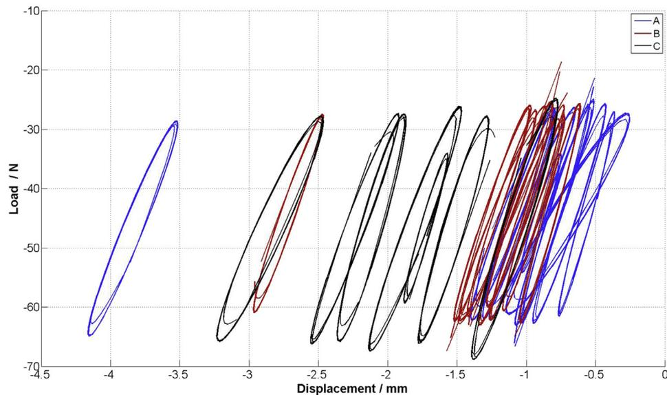
**Figure A.1** Five-cycle load–displacement curves of all specimens in Group A (blue), Group B (red) and Group C (black) at the time point after 5000 cycles.
