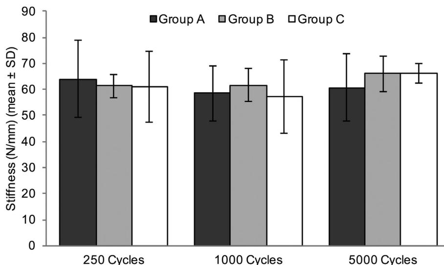
**Figure 3** Diagram representing construct stiffness after 250 cycles, 1000 cycles and 5000 cycles in terms of mean and SD. SD = standard deviation.
