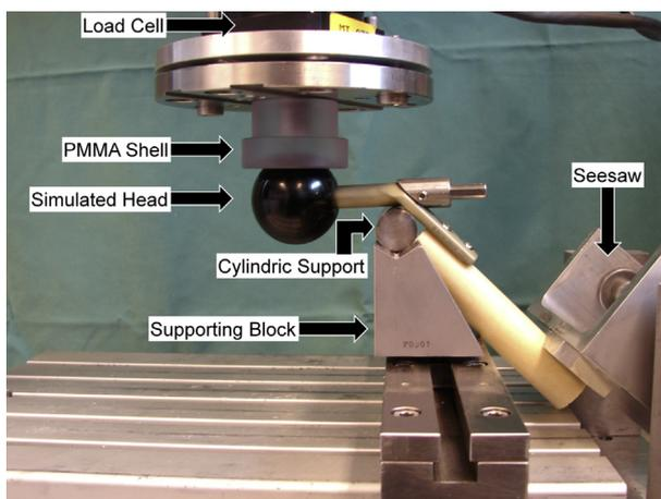
**Figure 2** Test setup with a specimen mounted for mechanical testing.
