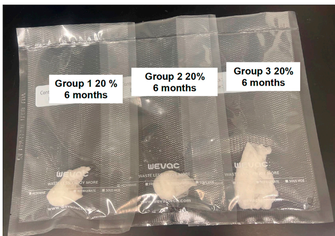
Figure 2. Soaked gauze in vacuum-sealed commercially available plastic packets packaged using a food vacuum sealer for storage. Treatment groups from left to right: Group 1—autoclaved glass bottles that were autoclaved again following solution preparation; Group 2—autoclaved glass bottles that were not autoclaved again following preparation and addition of saline; and Group 3—non-autoclaved plastic bottles that were not autoclaved following preparation and addition of saline.
