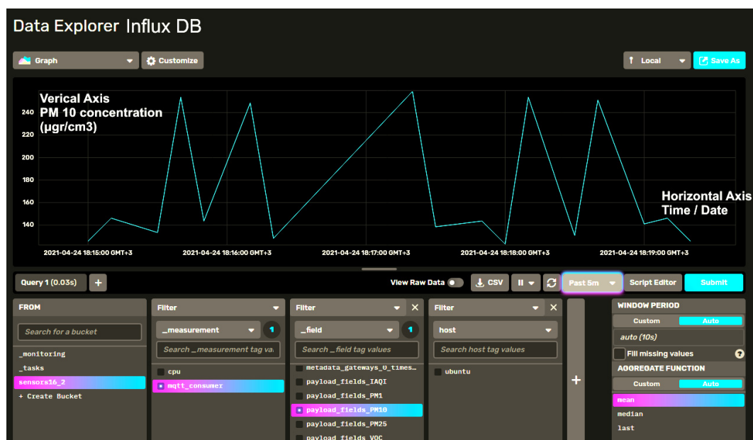
Figure 12. InfluxDB data Explorer visualizing PM 10 accumulated data in time series for the depicted time interval of 5 min.
