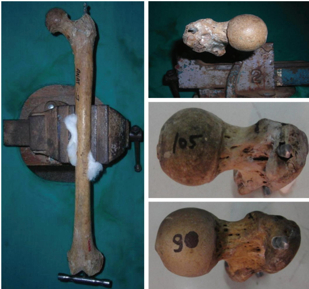
FIGURE 1: Showing femur mounted over frame with remur passed through intercondylar area in medullary canal and Superior view of proximal femur with various exit points.
