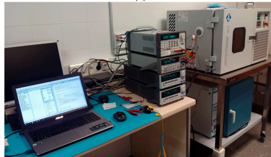
Figure 7. Measurement setup for the complete characterization of the LDO regulator: (a) block diagram of static (grey), transient load regulation (green) and transient line regulation (blue); and (b) experimental setup.
