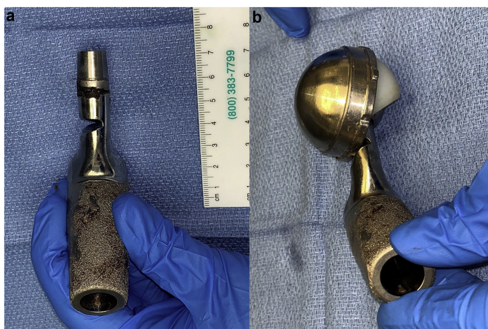
Figure 7. Femoral component notching (a) caused by impingement on the modular cobalt-chromium bearing in a dual-mobility construct (b).
