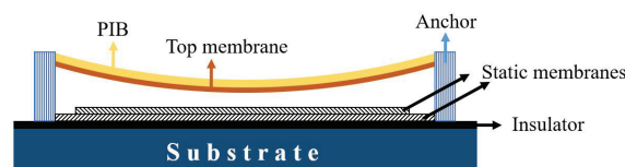
Figure 10. Schematic view of a CMUT sensor where the top flexible membrane is coated with a thin layer of PIB.
