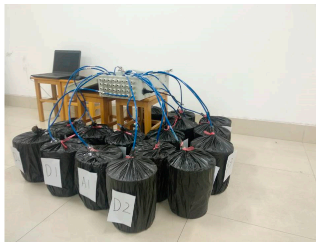
Figure 4. Self-volumetric deformation testing device for concrete.
