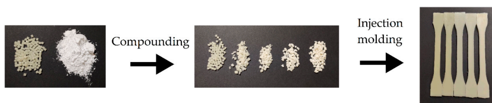
Figure 6. Processing steps carried out to prepare the poly(3-hydroxybutyrate-co-3-hydroxyhexanoate) [P(3HB-co-3HHx)]/hydroxyapatite nanoparticle (nHA) parts; from left to right: as-received P(3HB-co-3HHx) pellets and nHA powder, compounded pellets of the nanocomposite, injection-molded parts.
