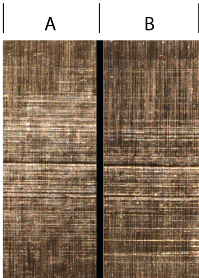
Fig. 2. Two consecutive segments of the tool mark. Note the similarity of the striations.
