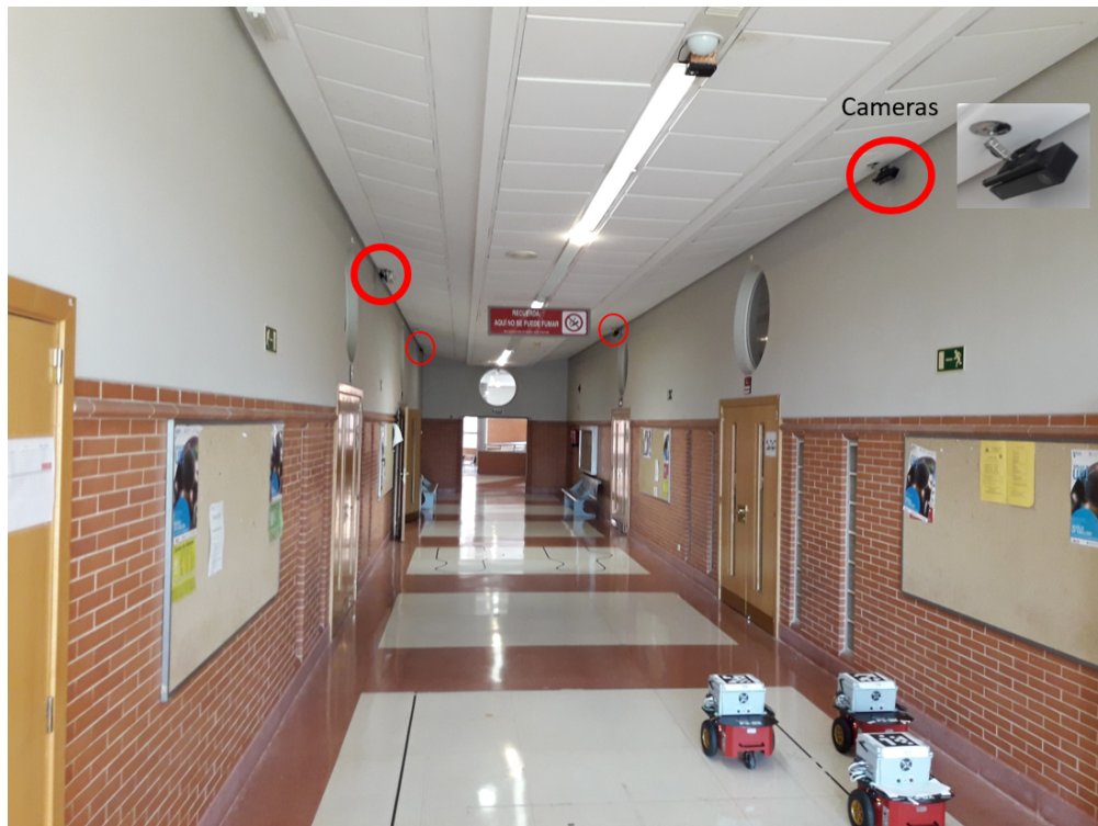
Figure 9. Picture of the working area with four Kinect 2 camera sensor and the formation of three P3DX robot wirelessly controlled by a miniPC.
