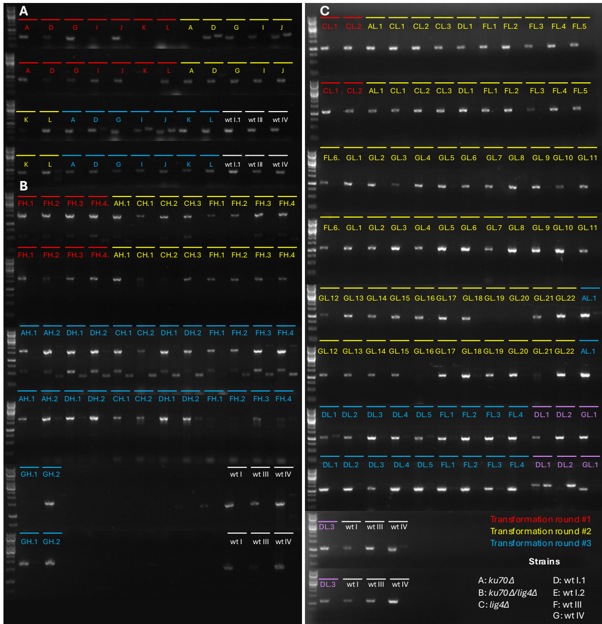
Figure S5: PCR results for cassette integration efficiency. Agarose gel electrophoresis images showing the PCR products of the adenine auxotrophy-based verified transformants. For each transformant, the upstream junction PCR products are loaded in the upper row, while the downstream junction PCR products are loaded in the lower row. In each row, for each transformant, the product of the primer pair binding in the ORF sequence is loaded first, followed immediately by the PCR product of a primer pair binding in the cassette in the adjacent right lane. A) Integration efficiency of the ENO1-SI system. A pooled sample of all transformants was used as template DNA for these PCRs. B) Integration efficiency of the HIS-FLP system. C) Integration efficiency of the LEUpOUT system. Transformants are grouped by transformation round and color-coded, with each sample labelled according to the strain code (A to G), gene editing system code (EN, H, L, or EP), and transformant number. The GeneRuler 1 kb DNA Ladder (Thermo) is loaded in the leftmost lane of each row.
