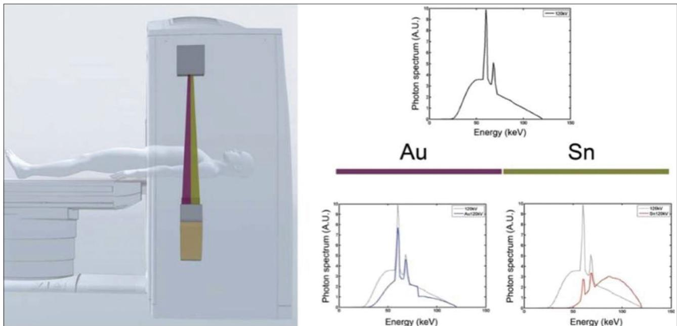
**Figure 1:** In twin beam DECT, two different filters Tin (Sn) and Gold (Au) are used to split the x-ray beam into two beams of different energies. The Gold (Au) filter, filters the high energy photons and produces a low energy beam while Tin (Sn) filter, filters the low energy photons and produces a high energy beam
