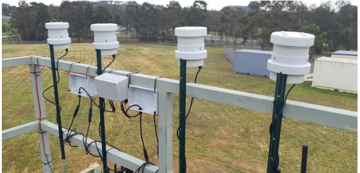
Fig 3. PM measuring devices under test at Department of Planning, Industry and Environment (DPIE) Campbelltown West air quality monitoring station (image: O. Price).
