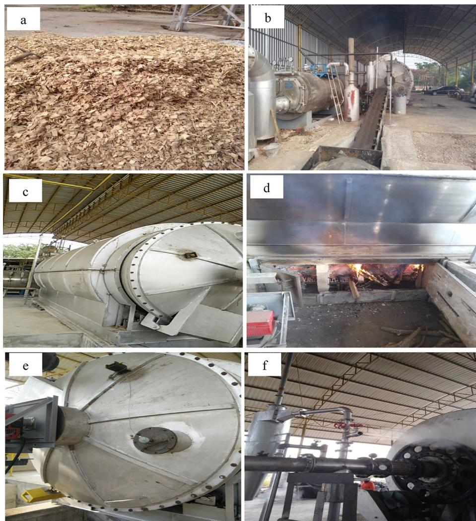
**Figure 6.** Activated carbon production system of batch intermittent rotary kiln: (a) sun dried eucalyptus wood chips, (b) conveyor belt, (c) rotary kiln, (d) wood stove, (e) thermocouples, and (f) pipe vent (25 mm diameter).
