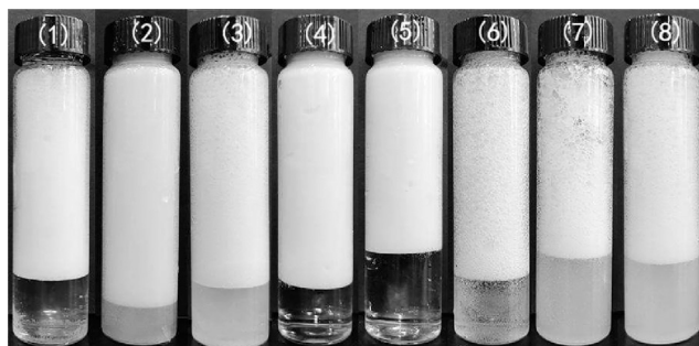
Figure 6. Drainage of foam at different C_{12}A concentrations
