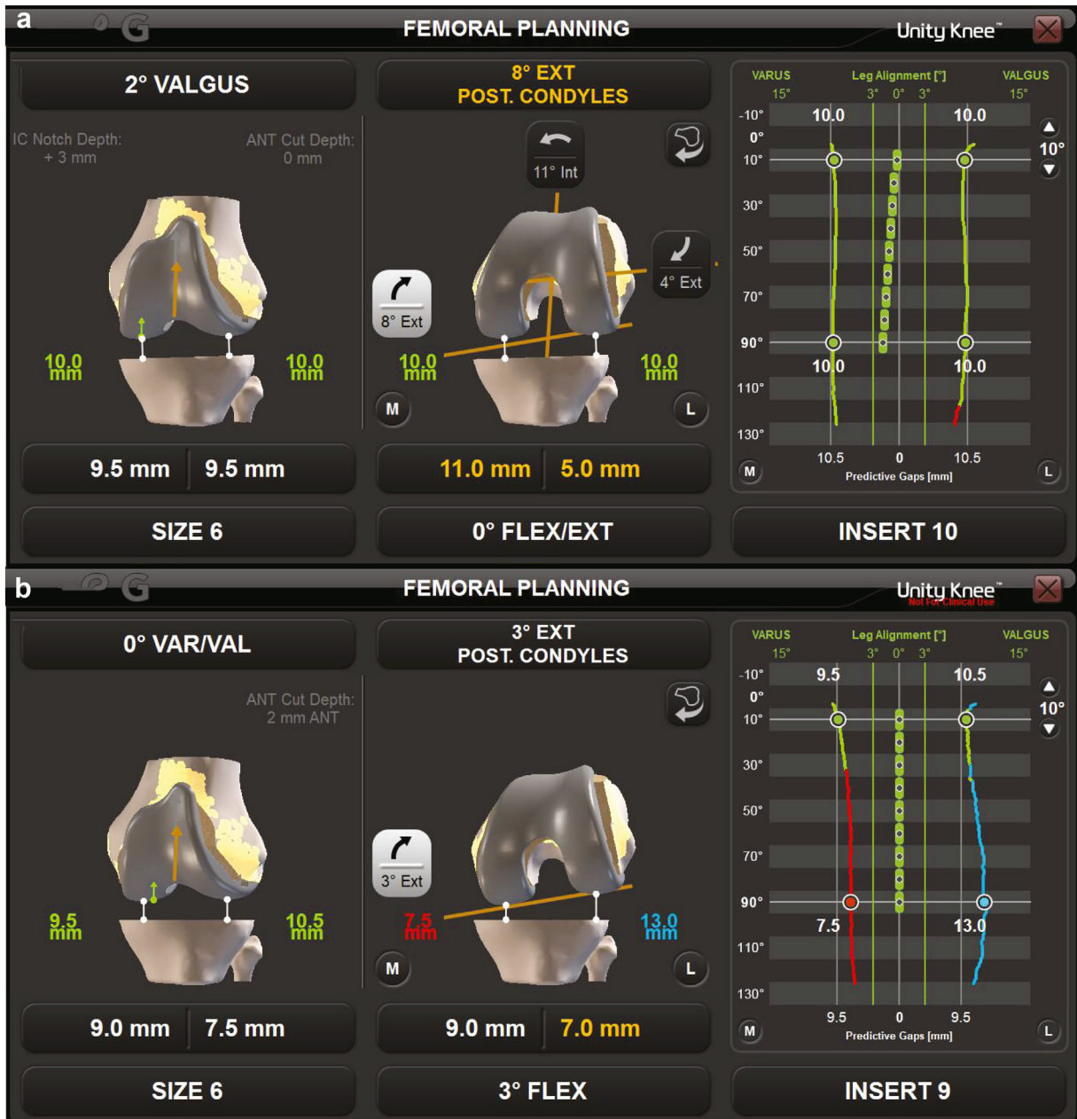
Figure 2. Femoral planning screens for pGB (a) and pMR (b). Femoral component adjustments are made using the computer system, and a predictive balance and laxity plan are provided throughout flexion.
