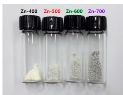
Figure 2. Photo images of the hydrogen generation powder samples prepared with zinc. Carbonate as a precursor at 400, 500, 600, and 700 °C in H 2 atmosphere.
