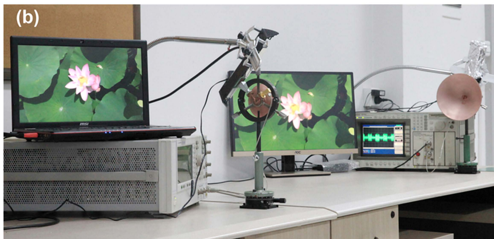
Figure 10. (a) The experiment setup of the dual OAM communication link. The l=+3 channel carries the square wave modulated millimeter-wave signal, and the l=-3 channel carries the HD video signal. (b) The experimental photo to demonstrate the successful transmission of two independent channels. The picture on the screen is extracted from the video, Copyright The Admission Office of Zhejiang University.
