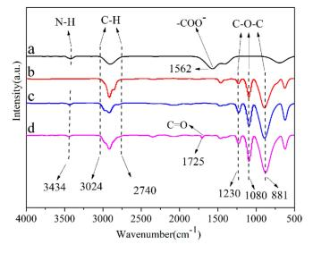
**Figure 2.** FTIR spectra of the (**a**) Ag nanoparticles, (**b**) POM, (**c**) POM/Ag nanocomposites, and (**d**) POM/Ag/MAH-*g*-POE nanocomposites.
