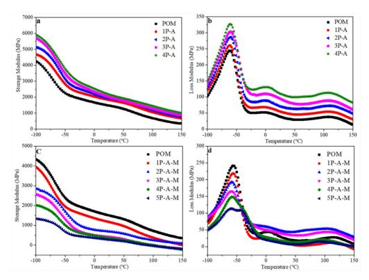
**Figure 8.** (a)Storage modulus diagrams and (b) loss modulus diagrams of POM/Ag nanocomposites; (c) storage modulus diagrams and (d) loss modulus diagrams of POM/Ag/MAH-g-POE ternary nanocomposites.
