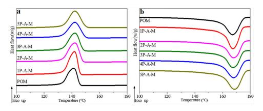
**Figure 5.** (a) Crystallization exotherms and (b) second melting end other ms of POM/Ag/MAH-*g*-POE ternary nanocomposites at a heating/cooling rate of 10 °C/min.
