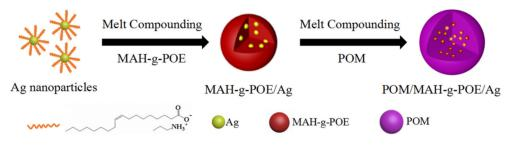
Figure 1. Synthesis procedure of POM/Ag/MAH-g-POE nanocomposites.
