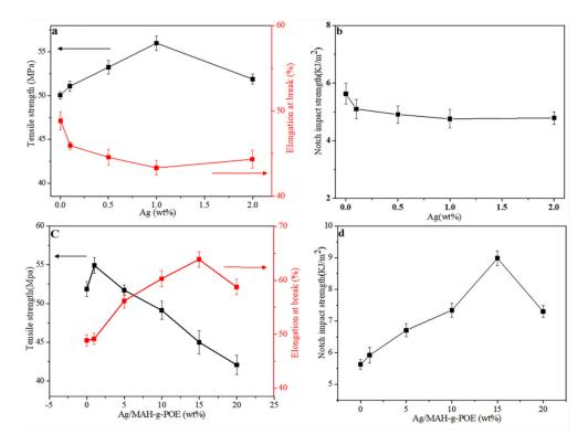
**Figure 6.** (a) Tensile strength and elongation at break and (b) impact strength of POM/Ag nanocomposites; (c) tensile strength and elongation at break and (d) impact strength of POM/Ag/MAH-g-POE ternary nanocomposites.
