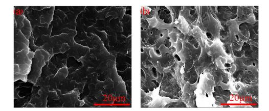
Figure 7. SEM of impact section of (a) 1P-A-M and (b) 5P-A-M.
