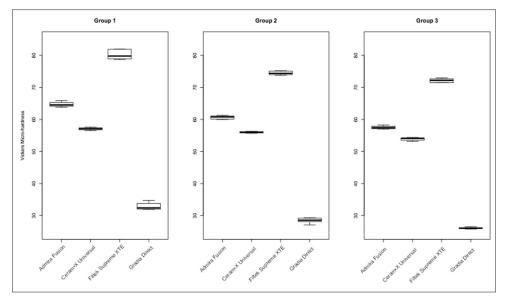
Figure 1: Box-plots for Vickers microhardness of material tested for each experimental group. Bold horizontal line represents median.
