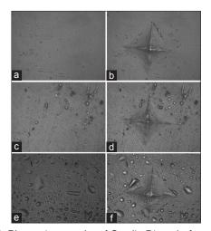
**Figure 5:** Photomicrographs of Gradia Direct before and after immersion in acidic drink for 1 and 7 days (×40). (a and b) Before immersion; (c and d) after immersion in acidic drink for 1 day, (e and f) after immersion in acidic drink for 7 days.
