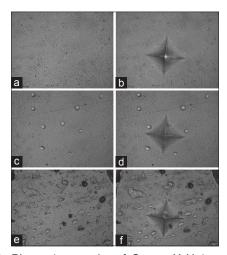
**Figure 3:** Photomicrographs of Ceram X Universal before and after immersion in acidic drink for 1 and 7 days (×40). (a and b) Before immersion; (c and d) after immersion in acidic drink for 1 day, (e and f) after immersion in acidic drink for 7 days.
