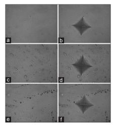
**Figure 2:** Photomicrographs of Admira Fusion before and after immersion in acidic drink for 1 and 7 days (×40). (a and b) Before immersion; (c and d) after immersion in acidic drink for 1 day, (e and f) after immersion in acidic drink for 7 days.
