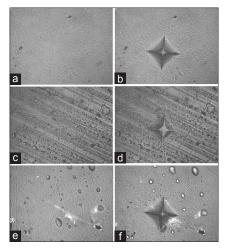
**Figure 4:** Photomicrographs of Filtek Supreme XTE before and after immersion in acidic drink for 1 and 7 days (×40). (a and b) Before immersion; (c and d) after immersion in acidic drink for 1 day, (e and f) after immersion in acidic drink for 7 days.
