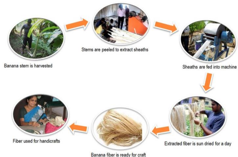
Figure 4. Mechanical separation of fibers from banana stems (adapted from [24]).
