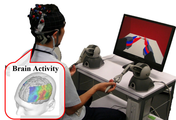
Fig. 1 Proposed method. We measured the user's brain activity using a f-NIRS brain activity measurement device during a simulation involving virtual robot surgery. The user moved the hand controller to manipulate the virtual arm
