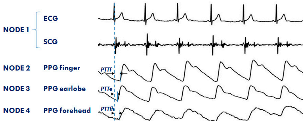
Figure 11. Example of signals from the 4 node configuration of the system aimed at investigating the PTT in different arterial sites: finger (PTTf), earlobe (PTTe), and forehead (PTTfh) by a multisite measurement of PPG.
