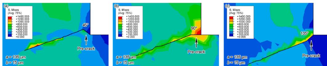
**Fig. 15.** Stress distributions and CPPs of the micro-notched specimens containing initial cracks at three different angles: (a) 45°, (b) 90°, and (c) 135°.
