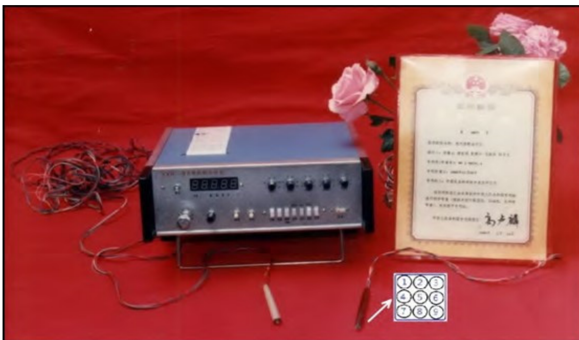
Figure 1. XXH-IIA Acupoint Diagnosis and Therapeutic Instrument used in this study; the white arrow points from the 1.5 cm diameter surface electrode probe to a diagram of the 9 sub-electrodes embedded in the probe head used to detect the area of lowest resistance within the acupoint; the probe on the left is the reference electrode; in this study an alligator clip electrode was used at the reference acupoint Wei-ben (used with permission).
