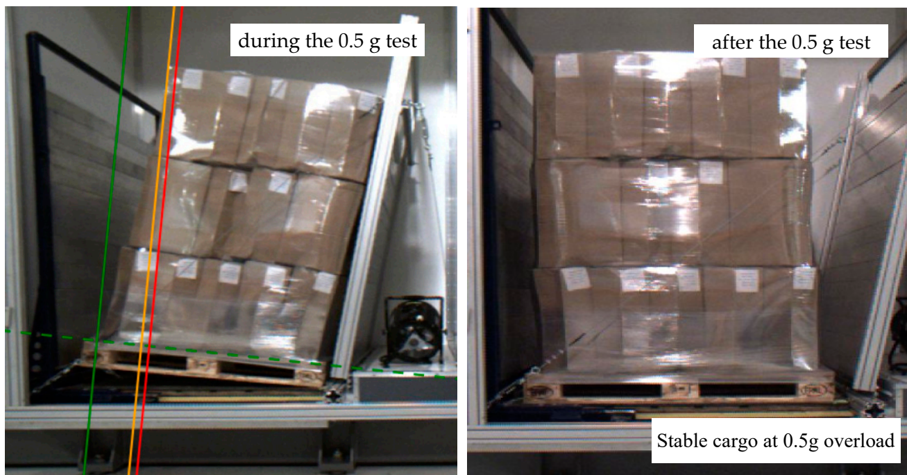
Figure 12. Cargo stability test at the set acceleration of 0.5 g.
