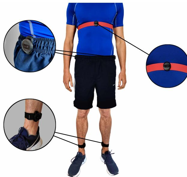
**Figure 5.** Subject wearing the Movesense IMU sensors on both ankles, hips and the chest.
