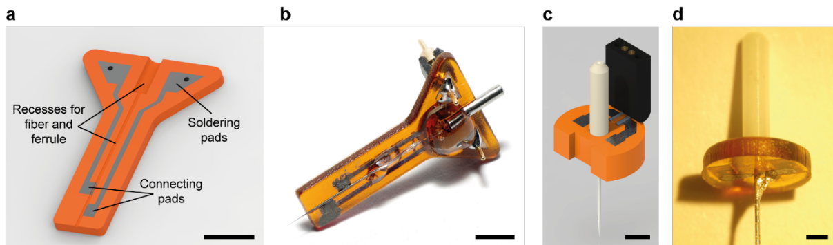
Supplementary Figure 2: Printed Circuit Board. (a) Rendering of a 3D printed PCB for acute implant; connection pads, soldering pads, and waveguide recesses are pointed out. Scalebar 5 mm. (b) Realized device with DIL pin connectors to interface with an electrophysiology headstage. Scalebar 5 mm. (c) Rendering and (d) device realized of a 3D printed PCB for chronically implantable devices with standard Omnetics connector for DAQ systems interfacing. Scalebars 2 and 1 mm.
