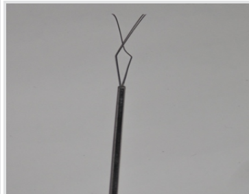
Figure 3: The breakage of a stainless steel lasso wire device that is used to shuttle sutures through the suture anchor insertion device.
