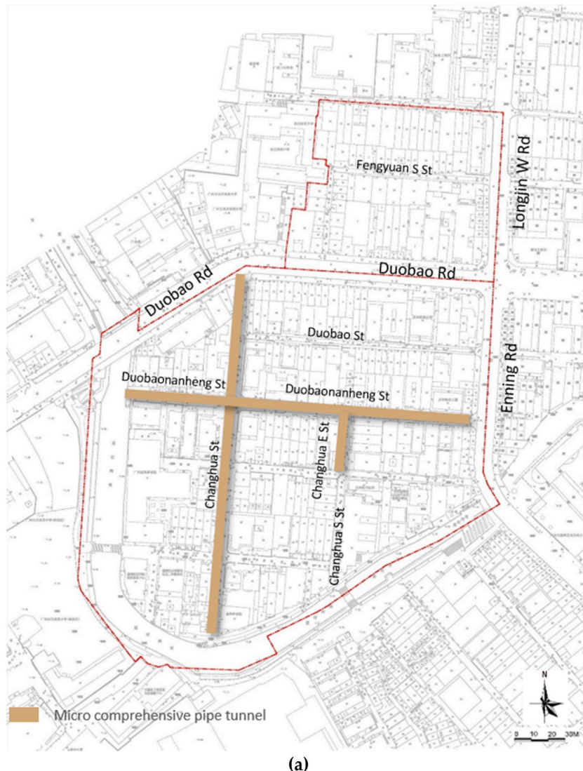
Fig. 4. Design of micro comprehensive tunnel systems. (a) System plan. (b) Street section.
