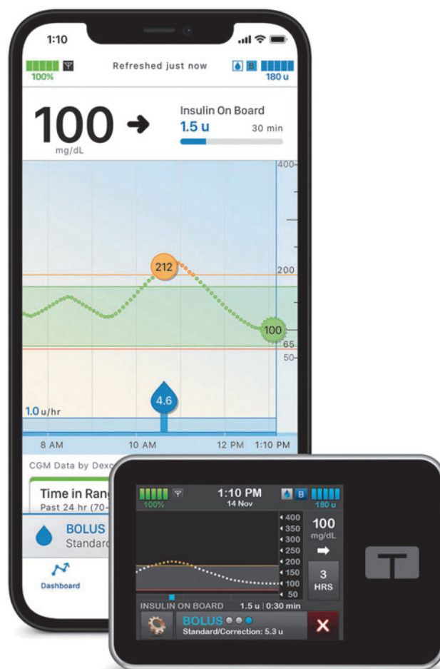
FIG. 1. The Tandem t:slim X2 insulin pump with Control-IQ technology. The hybrid closed-loop system consists of (1) the Tandem t:slim X2 insulin pump, (2) the Control-IQ technology glycemic control algorithm embedded in the pump, (3) a compatible iCGM, and (4) an optional smartphone app (iOS or Android) that allows for bolusing from a personal phone, acts as a secondary display for the pump, and uploads pump data automatically to the Tandem t:connect web application. iCGM, integrated continuous glucose monitor.
