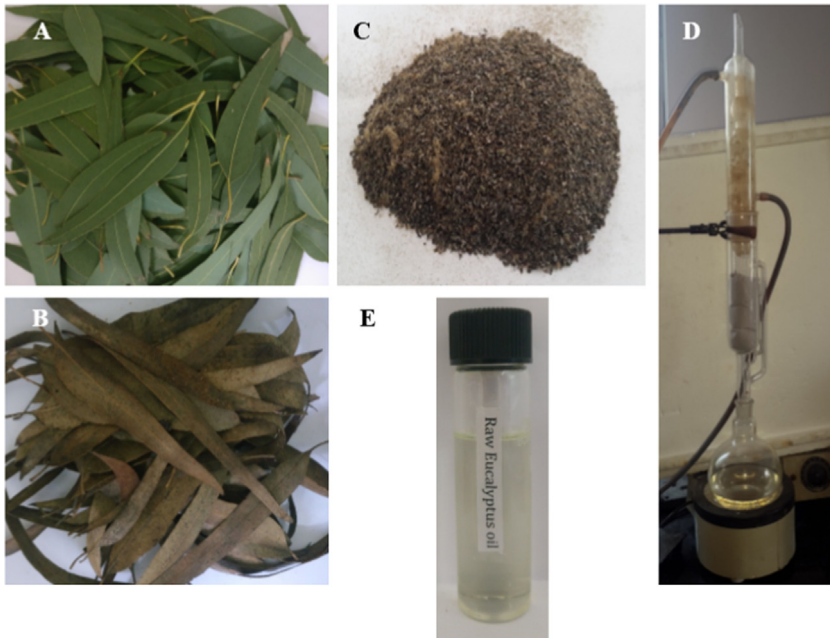
Fig. 1. Extraction of bio-oil from E.tereticornis through soxhlet extraction technique.
