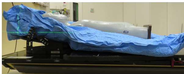
Figure 1. CIRS ATOM ® Model 705 anthropomorphic phantom in scanning position.
