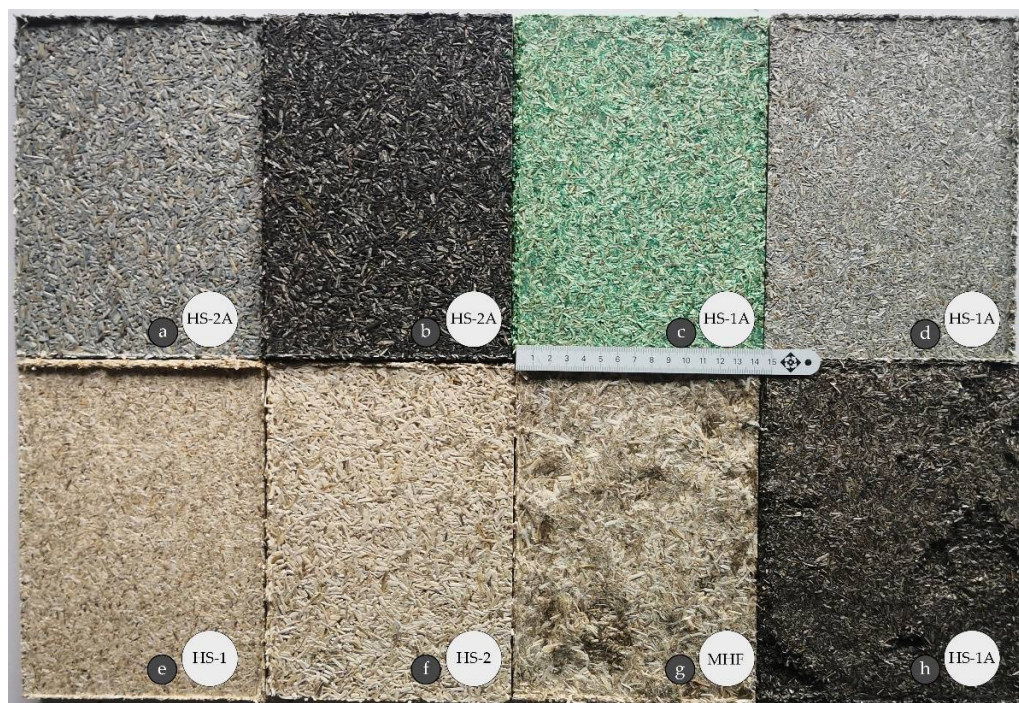
Figure 4. Surface view of board samples: (a) HS-2A sample with water-based wood coating applied on HS; (b) HS-2A sample with acrylic colorant applied during mixing process; (c) HS-1A sample with oil-based coating applied on HS; (d) HS-1A sample with water-based wood coating applied during mixing process; (e) HS-1 board sample; (f) HS-2 board sample; (g) MHF board sample; (h) HS-1A with oil-based coating applied on HS.
