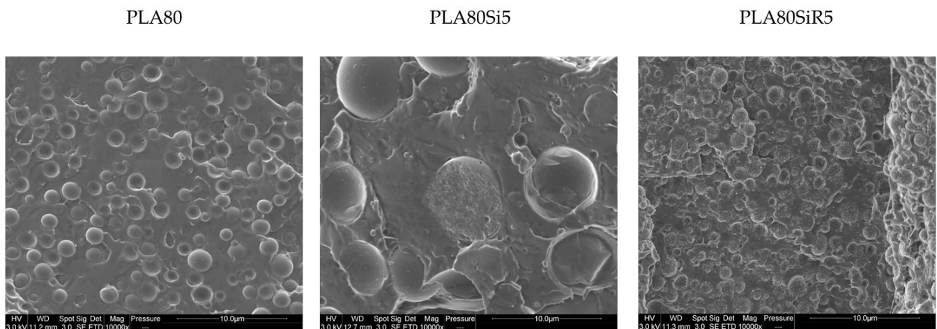
Figure 7. SEM micrographs of threads after extrusion for the PLA80, PLA80Si5, and PLA80SiR5. The samples were cut perpendicular to the direction of the thread.
