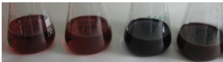
Figure 1 General view of AuNPs of discrete sizes: 10, 20, 30 and 45 nm.
