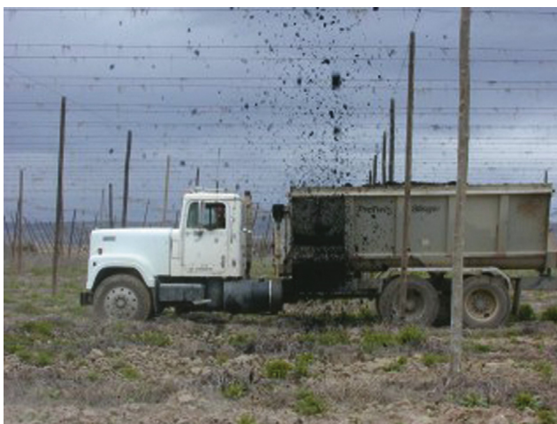
FIGURE 5.14 Land application of cake biosolids via a slinger in Solano County, California.
