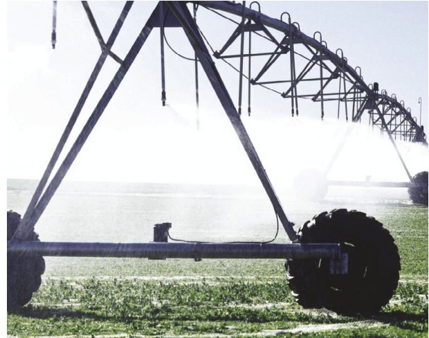
FIGURE 5.11 Application of secondary treated wastewater onto agricultural lands. This method is highly efficient at conserving water and has been shown to improve the fertility of soils. Due to the presence of pathogens in wastewater, and the nature of these land application systems, there are high concentrations of bioaerosols generated. Currently, however, there is little epidemiological and microbial risk assessment information available to determine if there may be health concerns for populations living in the vicinity of such operations, though there is a growing base of information on the concentration and types of pathogens found in these bioaerosols.
