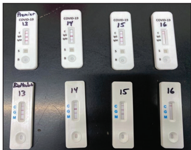
FIGURE 1. Premier Diagnostics (top row) and BioMedomics (bottom row) lateral flow assays. Cartridges 13–15 illustrate positive results for both IgG and IgM, whereas cartridge 16 illustrates negative results for both IgG and IgM.
