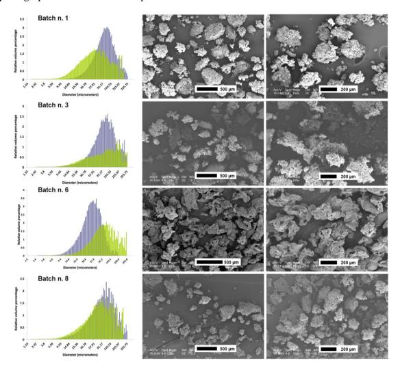
On the contrary, particles of the other batches appear to be formed by the aggregation of smaller spherical particles that probably occurred during the impact with the gelation solution (Figure 5). This
