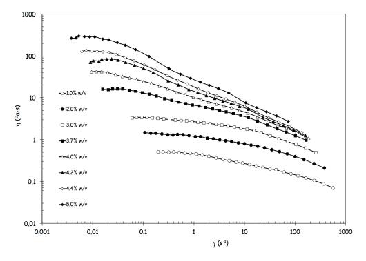
Data of Figure 2 clearly show how the shear thinning behavior becomes increasingly evident with increasing alginate concentrations, because the increase of viscosity is more pronounced at the lower shear rates [14]. In parallel, the critical shear rate marking the transition from the upper Newtonian plateau to the shear thinning region shifts at lower values (Figure 2). The flow behavior can be satisfactorily described with the Carreau-Yasuda equation (Equation 1),
