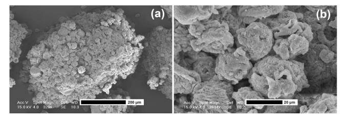
Counterintuitively, in this specific case, the larger particle size corresponded to the higher angle of repose. Generally, it is believed that the larger is the particle size, the better is the flowability but this was not the case. Obviously, the particle size and distribution are not the only characteristics that influence the flowability and particle morphology, porosity, and surface area should be taken into
