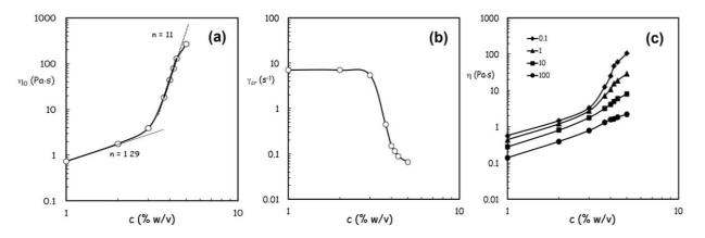
The pronounced drop in the critical shear rate c occurring above 3% w/v underlines how much the extension of the upper Newtonian plateau is confined at very low shear rates at higher alginate concentrations owing to the remarkable role played by inter-polymeric associative interactions on the rheological properties of concentrated FSs.
