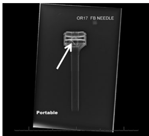
FIG. 2. Portable radiograph showing needle in trocar head (white arrow).
