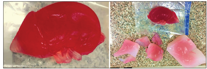
Figure 4: Final kidney phantom after it has ejected from the mold
